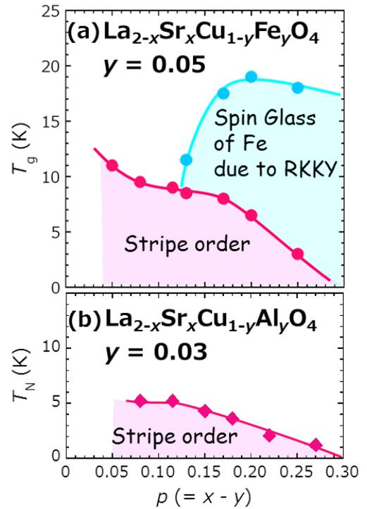
Fig.: (a) Hole concentration per Cu,  $p$ , dependence of  $T_g$ , defined as local maximum in magnetic susceptibility, for  $\text{La}_{2-x}\text{Sr}_x\text{Cu}_{1-y}\text{Fe}_y\text{O}_4$  with  $y = 0.05$ . (b)  $p$  dependence of the magnetic transition temperature defined by  $\mu\text{SR}$ ,  $T_N$ , for  $\text{La}_{2-x}\text{Sr}_x\text{Cu}_{1-y}\text{Al}_y\text{O}_4$  with  $y = 0.03$ .
